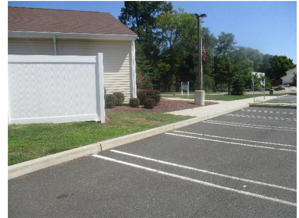
Parking spaces can be replaced with porous asphalt to capture and infiltrate stormwater. The installation of rain gardens adjacent to the building can capture, treat, and infiltrate roof runoff. A preliminary soil assessment suggests that the soils have suitable drainage characteristics for green infrastructure.
