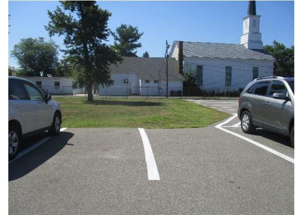
Parking spaces can be replaced with porous asphalt to capture and infiltrate stormwater. A bioretention system can be installed to capture, treat, and infiltrate parking lot runoff. A preliminary soil assessment suggests that the soils have suitable drainage characteristics for green infrastructure.
