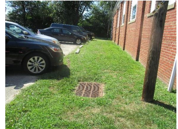
Parking spaces can be replaced with pervious pavement to capture and infiltrate stormwater. Bioretention systems can also be installed to capture, treat, and infiltrate runoff. A preliminary soil assessment suggests that the soils have suitable drainage characteristics for green infrastructure.
